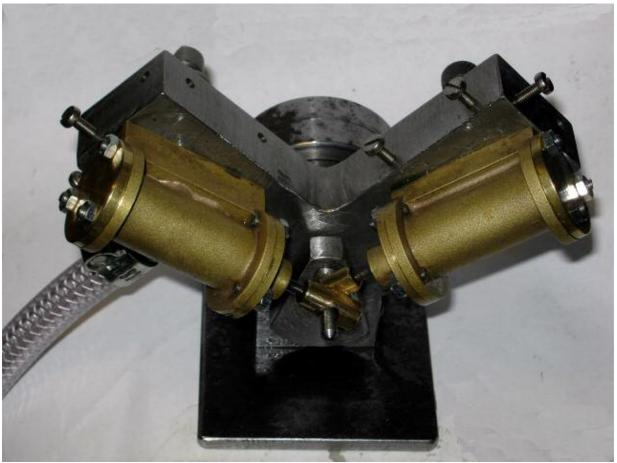
The parts were mounted and the engine was connected to my friends air compressor. It was a bit stiff to begin with, but after running at around 3 bar for some time it was possible to get the engine running as low as 1 bar, even if there were no packing in the piston groove or gaskets or gland packing. It seems that a
