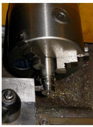
The piston rod big end bearing was made from some left over pieces of square brass. The brass was mounted in the 4-jaw and turned to a little over 6mm diameter for a length of nearly 6mm. The work was then transferred to the milling machine and the hole for the crankpin drilled.
