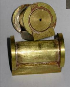
The steam ports were marked out and drilled and the hole for the pivot pin drilled and tapped M4. There were still remains of the
