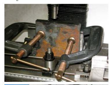
After milling top and bottom the work was transferred to the lathe and mounted in the 4-jaw. The side where the steam ports will be drilled was faced
