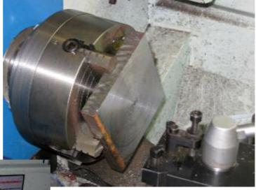
drill a bit deeper before opening up with the 2.5mm again. I managed to drill all the long steam passages without breaking the drill. If I wasn't able to drill the long steam passages successfully, there wouldn't be a V-twin, so I started with the standard.
