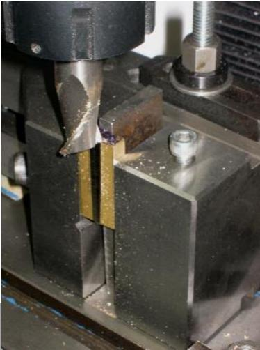
milling cutter to mill the flange to a close fit on the port block/cylinder. After cleaning and fluxing, the parts were silver soldered together and pickled for half an hour in citric acid – left photo.
