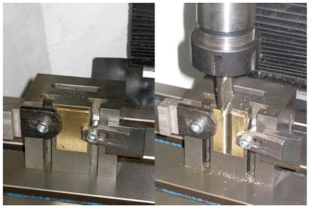
depression in the brass flat. I used a T-slotted box angle plate to clamp the brass flat and a 15mm diameter slot drill to mill a groove around 1mm deep. This approach gave much better results during silver soldering.
