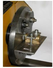
The two portholes were drilled 2mm to a depth of around half the distance between the cylinder bore and the portface. The cylinder was held at an angle in the vice and the steam passages were drilled from the edge of the cylinder end into the 2mm hole drilled from the portface. Before drilling I used a small slot drill to mill a small flat for the drill to start from.
