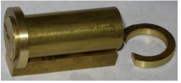
flat. The pieces was then cleaned, fluxed and silver soldered. After silver soldering the cylinder was pickled in citric acid.
