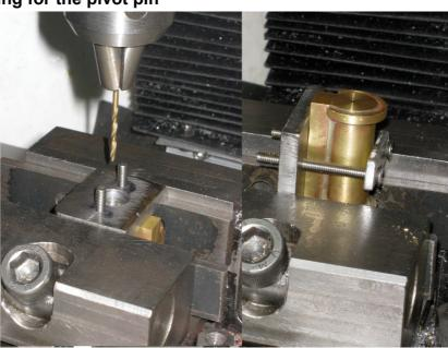
with a countersunk hole in the middle with M4 tapped holes on each side. The jig was milled on each side to make both sides flat and parallel. This way I could clamp the cylinder port face to the jig and place the jig on parallels in the vice and drill for the pivot pin and tap the hole M4.
