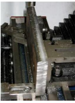
After milling the long sides of the sine table and removing the corners, the work was mounted flat on the milling table with a couple of parallels underneath (see right photo). Now all sides could be milled getting the sides of the table parallel and the corners square. I used a rotating carbide file on the long sides due to some hard spots left after the flame cutting.
