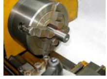
them to run true. At each end a 6.9mm hole was drilled to a depth of 12mm and tapped M8.
