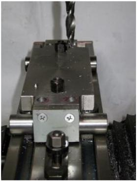
The holes for clamping the round bars to the end pieces were drilled 5mm diameter and counter bored. The last operation was to mill the bottom of the end pieces at an angle – see right photo.
