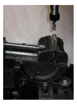
Below is a photo of the sine table in use for milling a 60T worm wheel for a rotary table.
