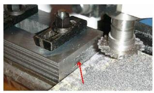
After the slots were milled I clamped the bottom piece to the milling table and used a dial test indicator to make sure its sides were parallel to the milling table. I then used one 8-mm end-mill to mill the sides of the slot parallel to each other. The end-mill was rather dull when I finished.
