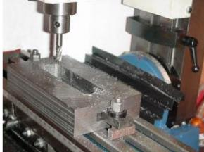
The last cuts on the bottom part were made after the centre slot was milled. I added another clamp (see the picture to the right) and milled two 6-mm deep and 6-mm wide slots along each side. Since these were cut without moving the workpiece, the slots should be parallel to each other. These slots will act as a guide for the movable jaw.
