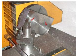
The bottom part has a slot for the M 12 Allen screw that tightens the movable jaw, so the next operation was to drill 4 holes. One 12-mm hole in each corner, I then used a hacksaw to cut the slot roughly to size (right picture).
