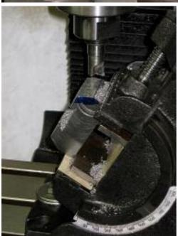
To make a tool-holder I used a piece of mild steel about 28 x 66 x 47 mm, the work was squared in the milling machine and the position of the dovetail was marked out. A recess was milled first using a slot drill, see left photo.
