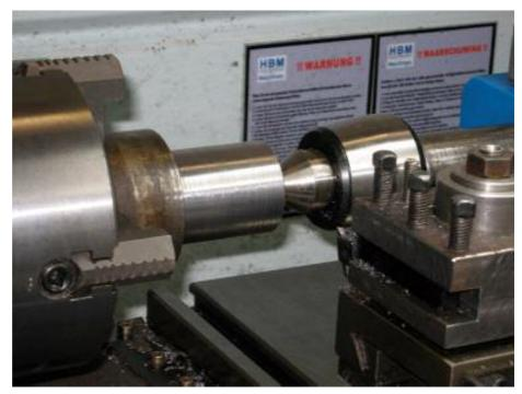
to the base by four M8 Allen screws. I also used Allen screws to clamp the base to the cross slide, and had to mill a groove in the widest part of the column to be able to get a key into the socket and turn the
