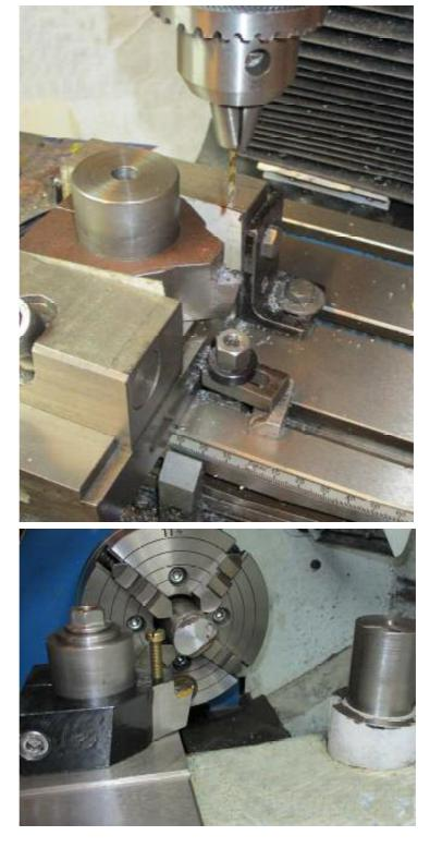
I also drilled a 5mm hole and tapped M6 for a height adjustment screw.
