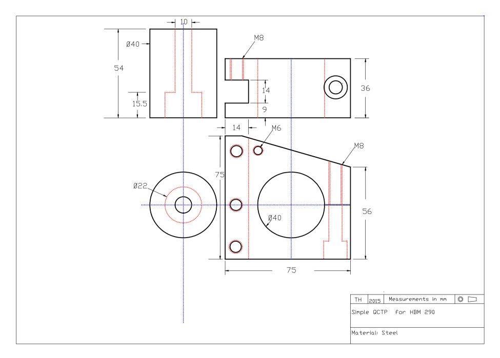
Toolpost for HBM 290 lathe -15-
