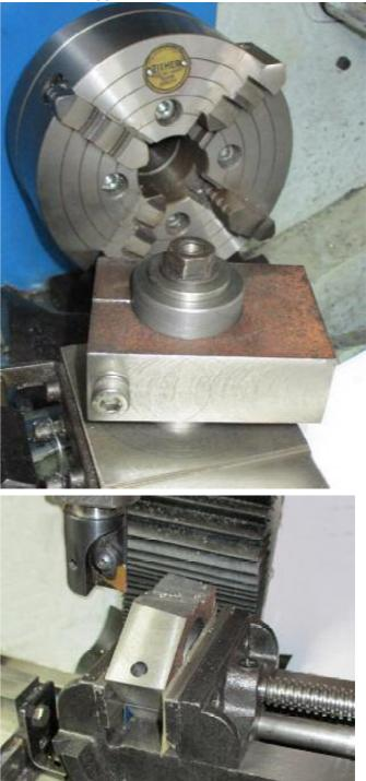
The tool-holder was mounted in the milling vice and I milled a step for the tungsten carbide insert. The insert was put in place and the hole for the clamping screw marked out. I didn't have a M2.5 screw so I tried to put a countersunk M3 Allen screw through the hole in the insert, and the hole was wide enough to let the screw pass. So I drilled a 2.5mm hole and tapped M3 – right photo.
