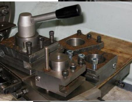
This photo show the toolpost and some of the tool-holders I made (and one I made earlier for my much smaller lathe).
