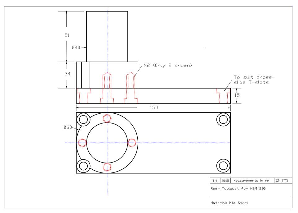
Toolpost for HBM 290 lathe -17-
