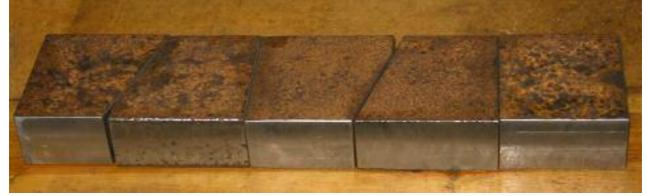
this way was twofold, I would get 5 toolholders instead of 4 and for 4 of them I would get more room when turning close to a revolving centre in the tailstock. The hacksawed parts of the 5 pieces were then milled before the centre hole was bored.
