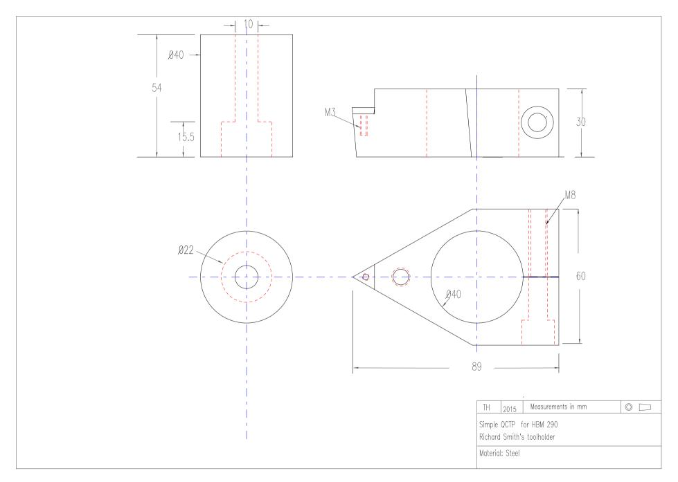
Toolpost for HBM 290 lathe -19-
