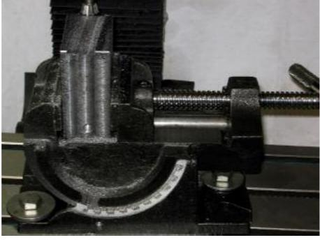
recess. This is so the HSS blade will seat well. On the opposite side I use a wedge shaped piece to clamp the HSS blade. I made two sizes of the wedge shaped piece so I can clamp two different sizes of HSS parting-off blades.
