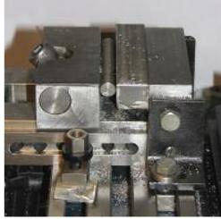
The collets are collapsed between the tapered brass piece and the taper in the front of the pin vise when you tighten the clamping nut.
