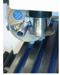
You can use a small hacksaw for the slitting process. Since the jaws of the chuck prevents the slitting saw from making the cut to the wanted length I used a hacksaw to get the slits to the length I wanted.
