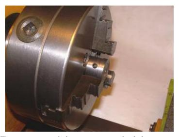
parted off for a total length of just over 16-mm. The next stop was made the same way, except that the large diameter was turned just under 20-mm. The stops was mounted the other way around in the 4-jaw, the jaws clamping on the small diameter of the disk stops. A small recess was turned on the front end and the hole for the set screw was drilled and tapped.
