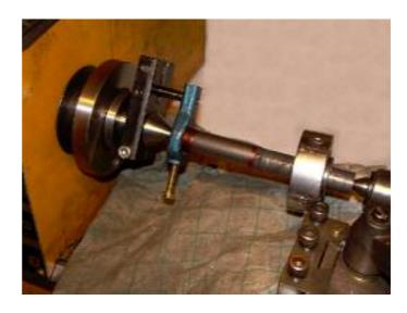
a close fit in the disk stops and a small flat for a set screw was milled. The total length of the carrier was adjusted so it almost reaches the front end of my smallest 80-mm 3-jaw chuck.
