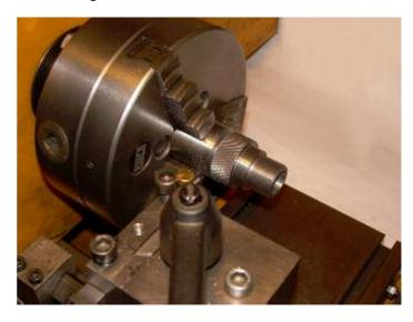
bar. I also turned a small 2-mm thick washer that just will pass over the threaded part of the nut. I insert this washer and tighten the nut before knocking the shank out of the lathe mandrel, this way the thread should not be damaged.
