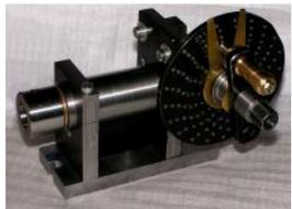
rings have been moved out of the way to show the keyway in the spindle. The spindle extends far behind the frame, so I guess I could shorten it quite a bit. I will thread the spindlenose 1 1/8-in. x 12 TPI and a register of 1 ¼ in., i.e. like the Myford 7 spindle nose.
