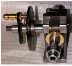
The spindle was case hardened so I used a carbide tipped tool to turn down the spindle nose and cut the thread. After I cut through the hard surface the material machined very well.
