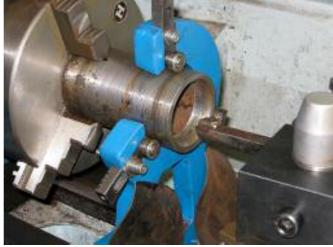
The next job was to drill a 8mm hole in each end piece and turn the end pieces so they fit into the recess turned in the pipes.
