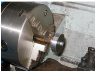
Each end piece was then chamfered so it would be ready to be welded in place - right photo.
