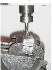
By tilting the vise I could use an end-mill to mill the one side of the slot left by the dovetail cutter a bit wider, to fit the wedge that press the parting blade towards the holder.
