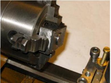
could be drilled 2.5mm and tapped M3. The 3mm holes in the *Bottom Cover* were countersunk on the side facing the *Bedplate*.
