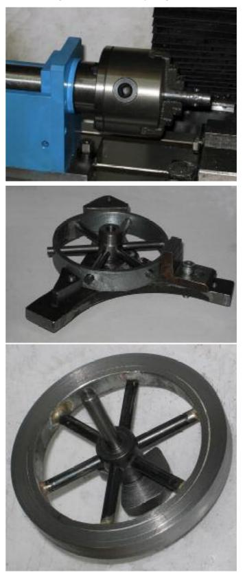
Loctite I used to secure the threaded rod had cured the ends were filed flush and the flywheel
