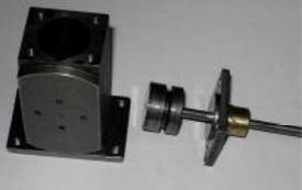
parted off side faced. The *Piston* with *Piston Rod* was then turned to a nice fit in the *Cylinder*. The *Piston Rod* was made from a piece of 1/8" free-cutting stainless steel, the M3 thread on the end was cut in the lathe.
