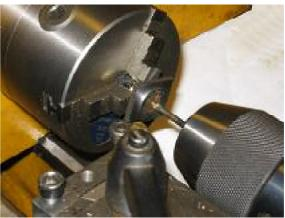
four 3mm holes 90 deg. apart in the Top Cover and used the Top Cover to spot the corresponding holes in the Cylinder top face. The four holes in the Cylinder were drilled 2.5mm and tapped M3.
