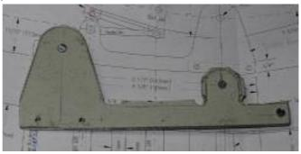
as a jig to drill corresponding holes in the second piece. The two pieces were bolted together using two small screws and then the other holes could be drilled through both pieces, as advised by Rudy. I used a file to file the parts to final dimensions.
