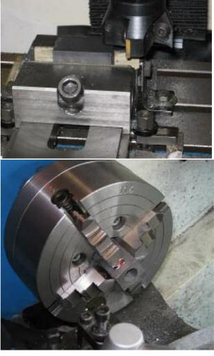
The work was transferred back to the milling machine and the *Valve Pivot Screw* and the four port openings were marked out on the *Port Face* at a PCD of 15mm. I used a 2mm drill for the ports and drilled them to a depth of just over 3mm.
