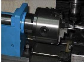
6mm dia. mild steel rod. The (over length) work was held in the 3-jaw on my indexing head and one side milled down 1mm for a length of just over 8mm. Then rotated 180 deg. and milled the same way. Then over to the lathe and the work was parted off to just over finished length, faced and centre drilled and drilled 2.5mm and tapped M3 for the *Piston Rod*. Then a 1.6mm hole was drilled from the front and into the hole for the gudgeon, and tapped M2.
