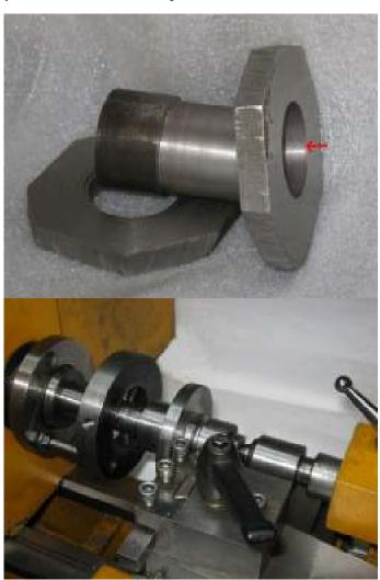
large pulley for the countershaft, but after a while a friend got me a large PolyV pulley that I could mount on the second hub. For the countershaft I used another piece of the 80mm square steel tube, but instead of Oilite bushes I used two 20mm Pillow Block ball bearings. The countershaft will rotate at a higher speed than the crankshaft. I also turned a small diameter PolyV pulley for the motor. I must find some material to make some belt and pulley guards.
