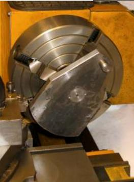
The crank was hacksawed from a piece of steel, a slightly undersize hole drilled and bored in the centre and a piece of 20mm bright steel rod (crankshaft) was pressed in. I also used a couple of so called "French keys" to make sure the rod would not move.
