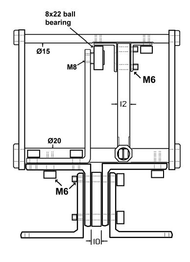
The sketch at the right shows the hacksaw as seen from the front. A friend gave me a 250mm dia. PolyV pulley that I used on a countershaft to reduce the speed of the 1500rpm motor
