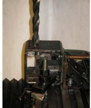
the work and the table) on my rotary table and mill the outer part circular.
