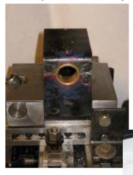
The photo to the right shows the crankshaft and bearing mounted on the base. A couple of oil-holes are visible on the top.
